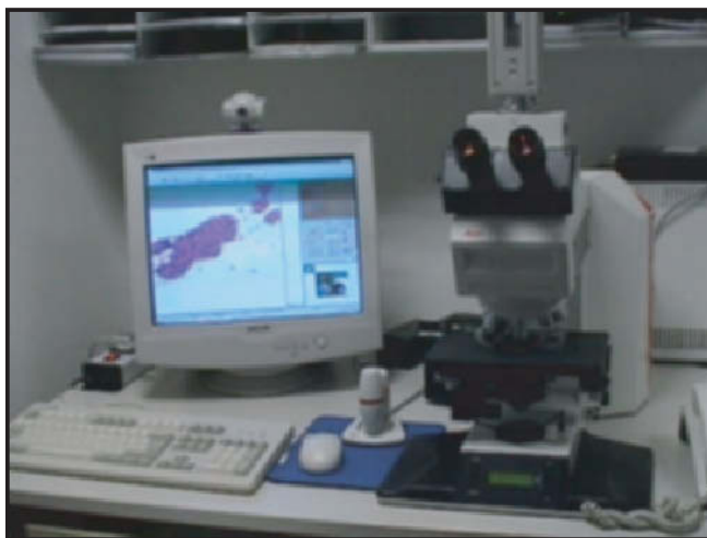
Figure 6.18 Telepathology. A telemicroscope (Leitz, Wetzlar, Germany) can be maneuvered by the pathologist on long distance communication. The diagnosis can be followed on microscopic image from the monitor and audiovisual communication with the pathologist is provided.
