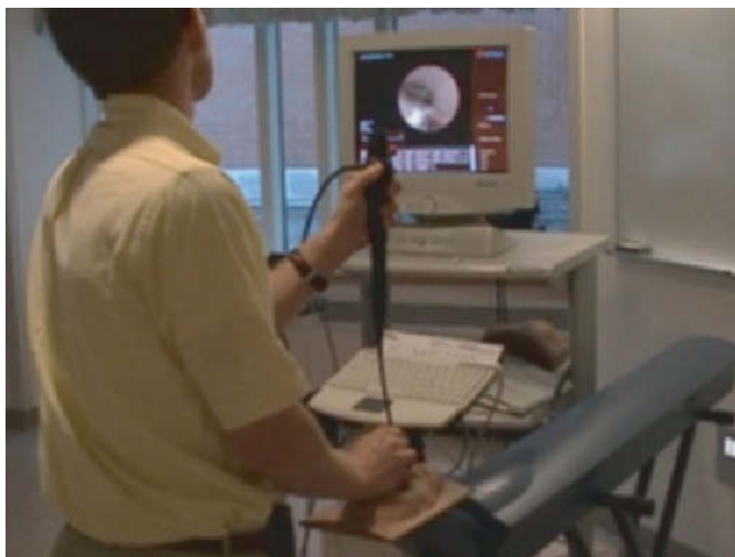
Figure 6.19 Virtual bronchoscopy trainer (Immersion™). The instrument is introduced via a mannequin's face and the simulator provides images of the normal and pathological bronchial anatomy. Additional features such as biopsy and transbronchial needle respiration can be performed in real-time simulation.
